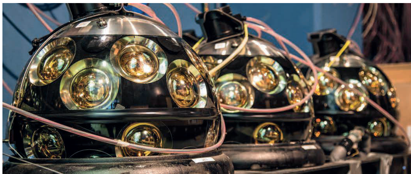
Cherenkov light sensors in the KM3NeT/ORCA neutrino telescope currently under development in the Mediterranean.
