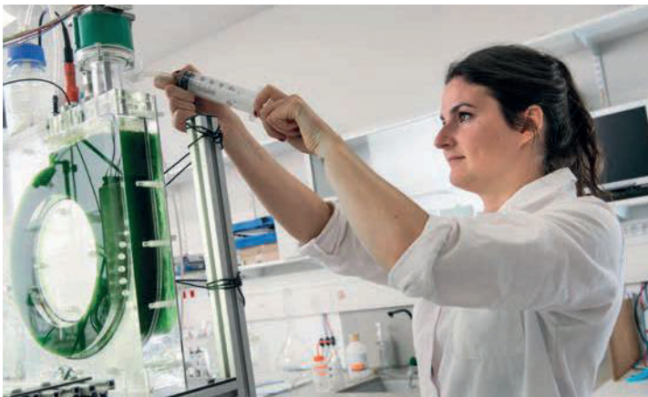
A pilot torus reactor in which a reference microalga is being cultured. © Jean-Claude MOSCHETTI / GEPEA / CNRS Photothèque
