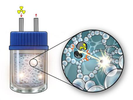
The scintillating aerogel is inserted into a scintillation vial. The gas to be analysed penetrates the vial and the aerogel via diffusion. Each decay emits an electron that interacts at very short distance with the "scintillating" nanoparticles that make up the aerogel. This results in a flash of light that is then detected, signalling the presence of the radionuclide. (© Zoé Dujardin)
